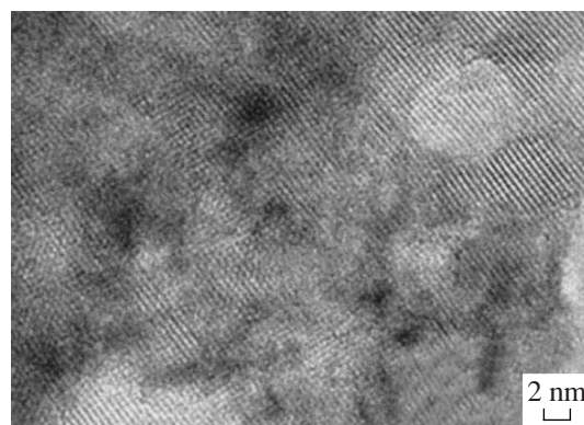
Fig. 2. Electron micrograph of the 5 wt % \text{CeO}_2 + 95 wt % \text{TiO}_2 support calcined at 500^\circ\text{C} .
